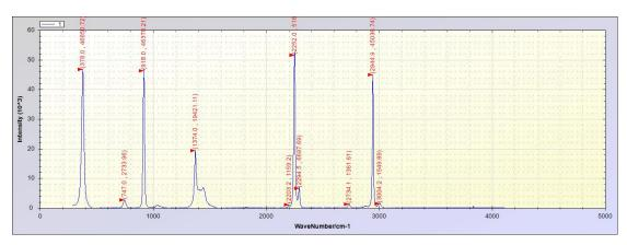
Figure 1 Raman spectrum curve test results; sample: acetonitrile, laser power: 130mW, measurement integration time: 4000ms.
